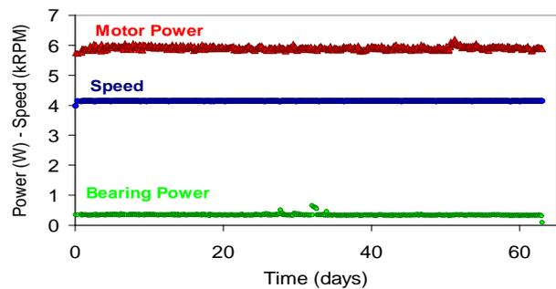
Figure 5. Data from the long-term durability testing of the MiTiHeart® LVAD
