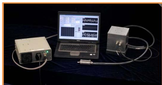
Figure 2. MiTiHeart<sup>®</sup> control system with battery pack and optional user-interface via PC
