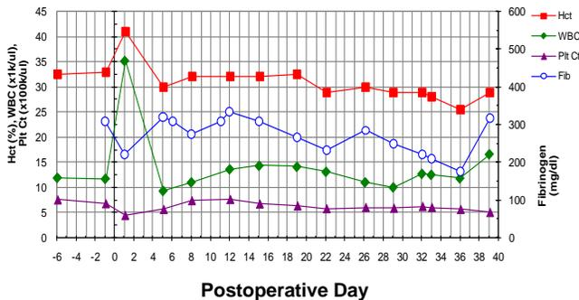
Figure 4. Typical hematological data recorded during long term chronic implant testing
